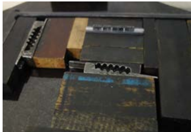
Type Lockup: Lead type is held in the case and braced out with wood blocks and quoins.
